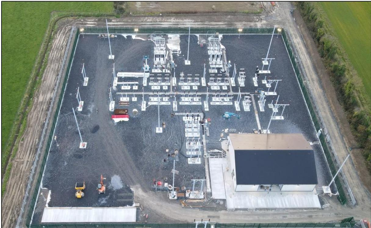
**Figure 4: Typical 110kV Electricity Substation**
